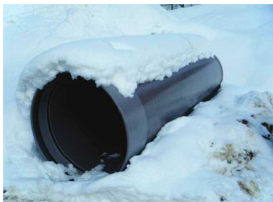
(埋設管FRPΦ 1100mm × 4m)
